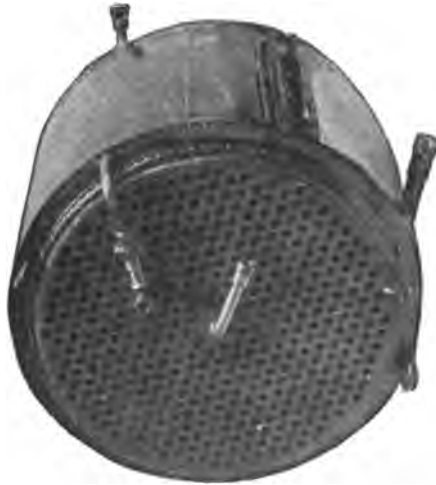
FIG. 148.—The Boiler used on the "Victor" Carriage, Top View, showing asbestos packing, steam and water connections, and method of riveting on the tube plates.
